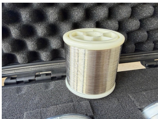
Close-up of a bare spool, Ø 0,025 mm wire
